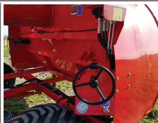
• Grain sampler; hydraulic controls; brakes
